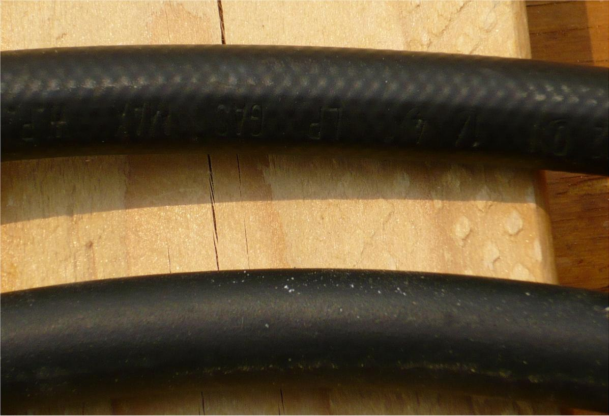
The long hose between the propane tank and the generator is marked. The 16" hose between the Pressure Regulator and the Carburetor has no markings.
