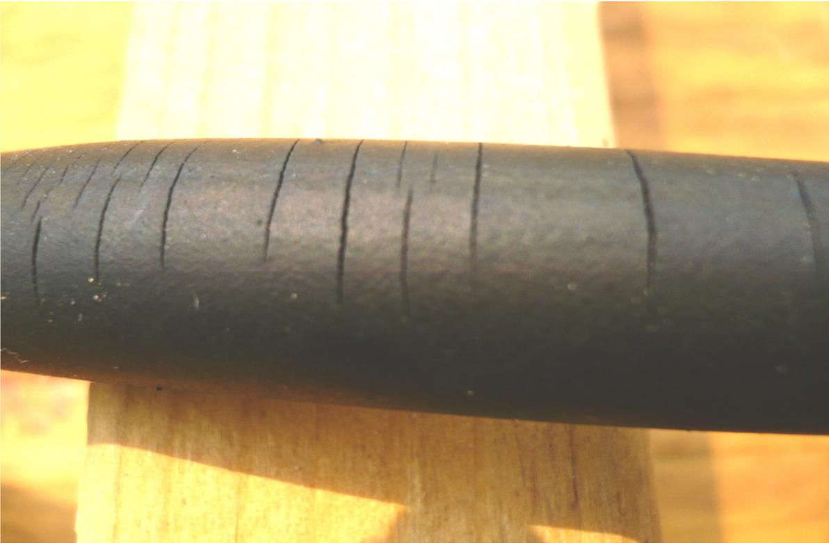
The end connected to the Pressure Regulator is completely cracked open.
