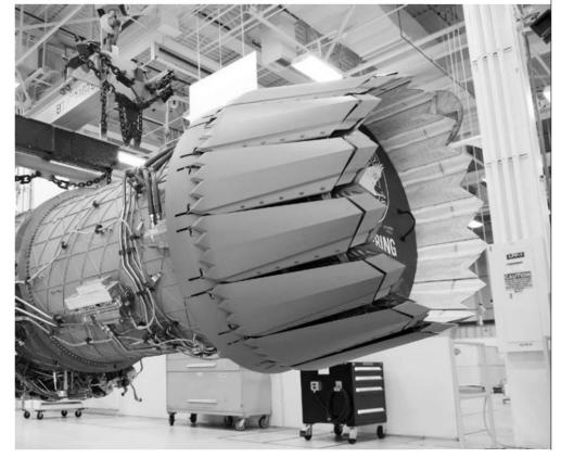
augmenters. Aft of the low-pressure turbine are thick, curved vanes that, when looking up the tailpipe, block any direct view of the hot, rotating turbine components. Fuel injectors are integrated into these vanes, replacing the conventional afterburner spray bars and flame holders. The vanes mask the turbine and contain minute holes that introduce cooler air.
