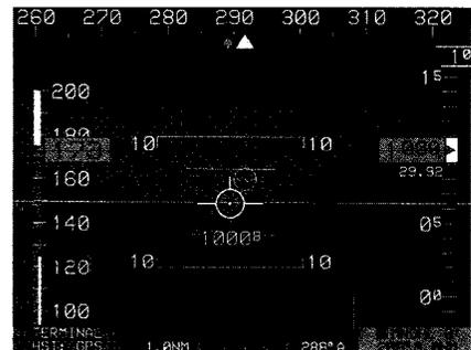
using HITS in Juneau, Alaska, on Mar. 31. It followed an optimized area navigation (RNAV) route through airspace that would be inaccessible with conventional avionics.
