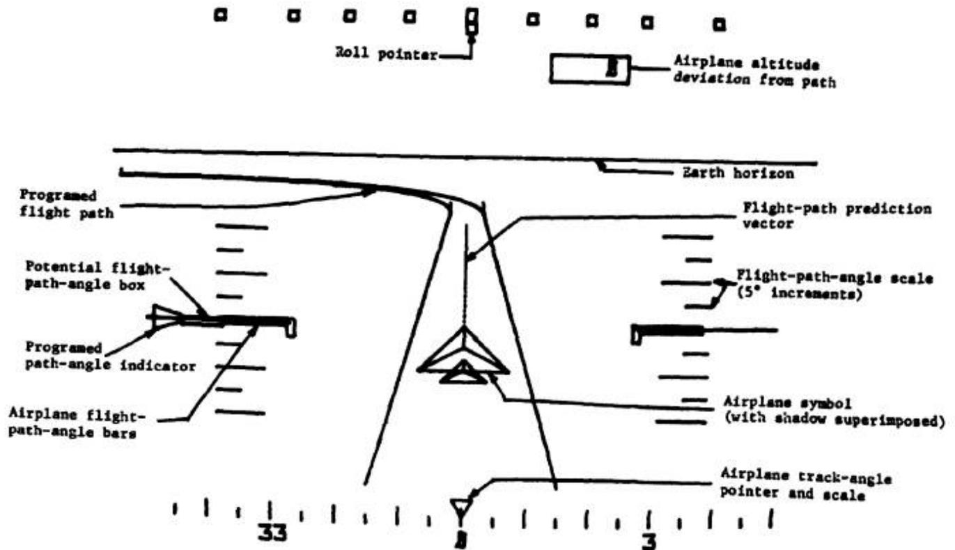
Figure 4.- The PITS contact analog display symbology.
