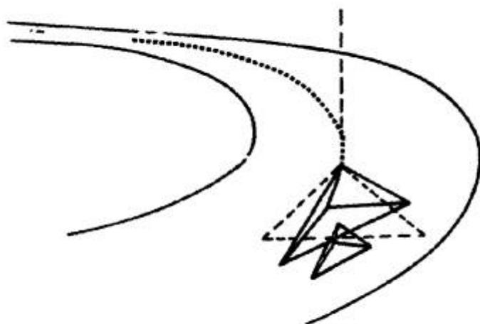
Figure 1.- Path, shadow, flight-path predictor, and airplane symbology.
