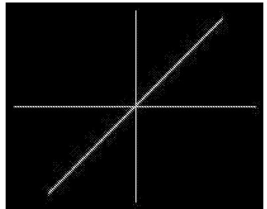
When the two sine waves are of equal frequency and 180 degrees out-of-phase you get a diagonal line to the left.
