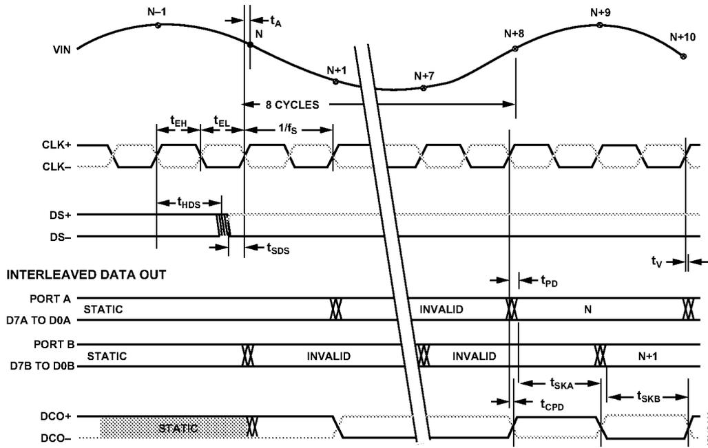
Figure 2. Timing Diagram
