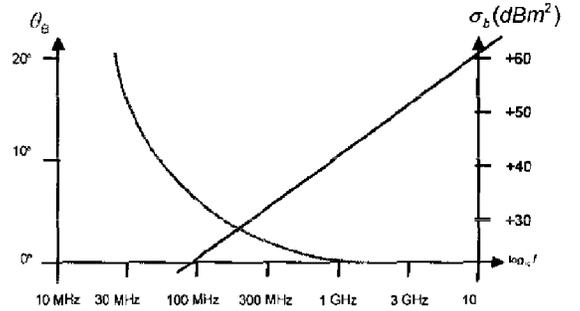
Fig. 4. Variation of forward scatter RCS and angular width of response ( $d = 10\text{m}$ ,  $A = 10\text{m}^2$ ).
