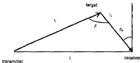
Figure 1. Bistatic radar geometry.
