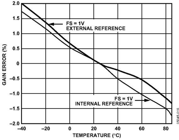
Figure 16. Full-Scale Gain Error vs. Temperature,
