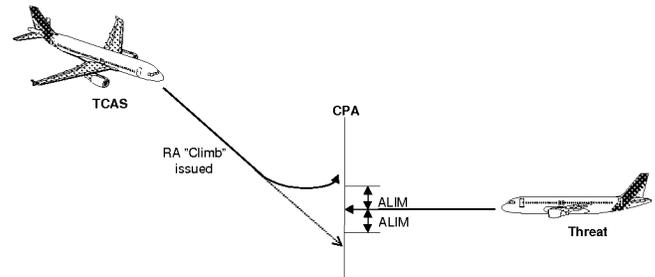
Figure 16. Selection of Noncrossing RA Sense
