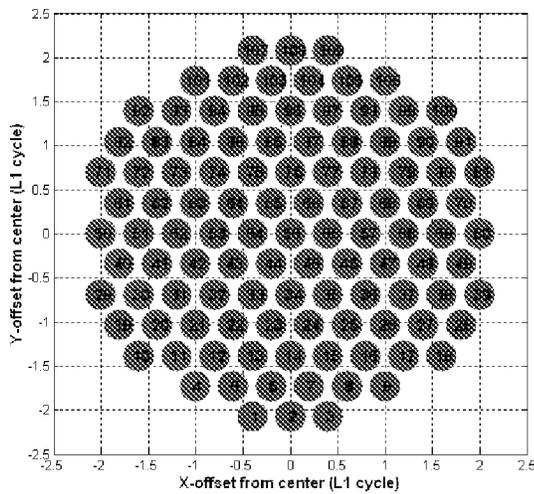
Figure 7 96-Element Phased Array
