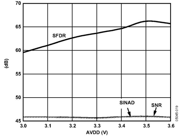
Figure 19. SNR, SINAD, and SFDR vs. Supply Voltage,
