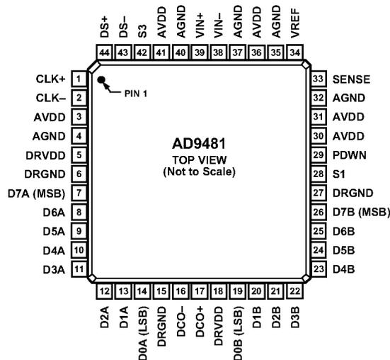
Figure 3. Pin Configuration
