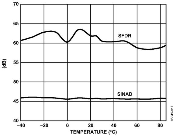
Figure 17. SINAD, SFDR vs. Temperature,
