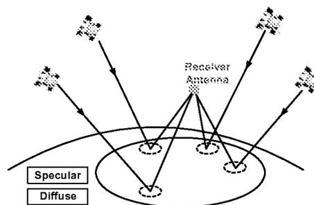
Figure 1 GPS Bistatic Geometry with Specular Reflection Points
