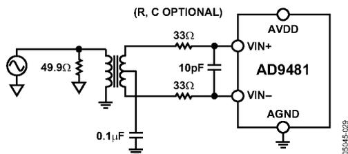
Figure 28. Driving the ADC with an RF Transformer
