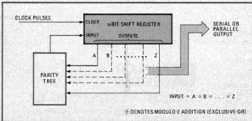
**1. Pseudorandom pulses . . .** In this linear-feedback shift register, some of the output ports are connected back to the input through an exclusive-OR circuit. Depending upon which output taps are fed back, a non-repeating sequence of any length up to  $2^n - 1$  binary words can be generated.
