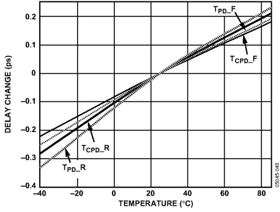
Figure 22. Propagation Delay Sensitivity vs. Temperature
