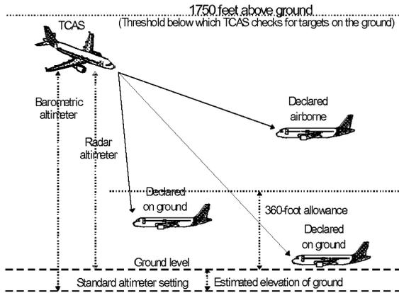
**Figure 14. Mode C Target on Ground Determination**
