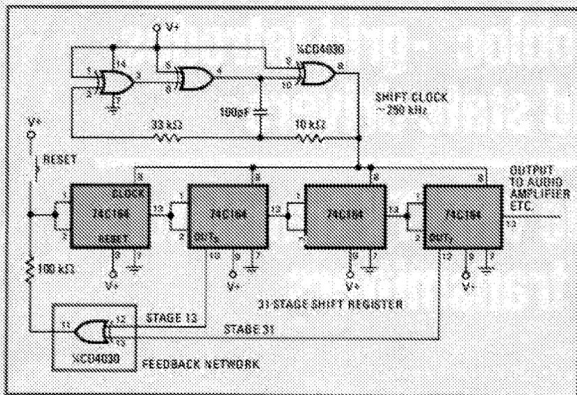
**2. . . generate noise . . .** This 31-stage linear-feedback shift register is arranged to produce a maximum-length pseudorandom bit sequence by connection of stages 13 and 31 back to input. Output bit stream, which can be taken from any port, constitutes a white-noise source.
