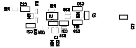
Figure 46. PCB Bottom-Side Silkscreen
