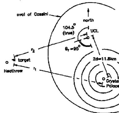
Fig. 10. Horizontal-plane geometry of Crystal Palace television transmitter and Heathrow. Indicated Oval of Cassini is the locus  $r_1 r_2 = 2 \times 10^8$  m.
