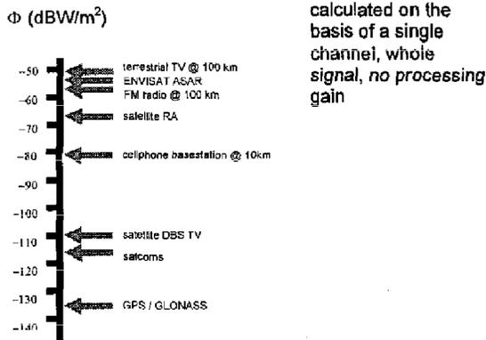
Fig. 5. Power density  $\Phi$  for various PCL illuminators.
