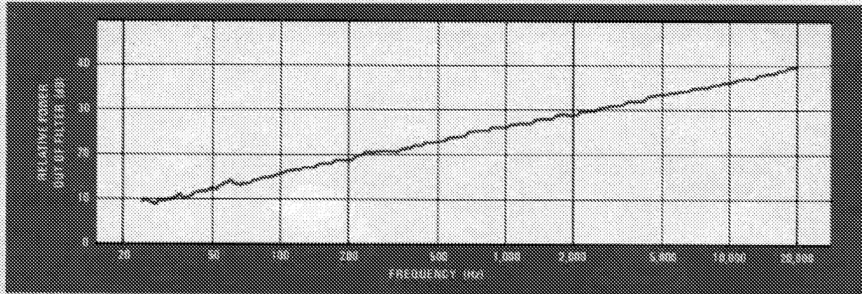
**3. . . like this.** The output power spectrum of the circuit in Fig. 2, measured directly at the output of stage 31, slopes upward because filter bandwidth is proportional to frequency. The slope of 3 dB/octave indicates white noise. Reference level (0 dB) was chosen arbitrarily.
