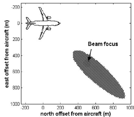
Figure 10 109-Element Beam Footprint (3dB contour from 500 m altitude)
