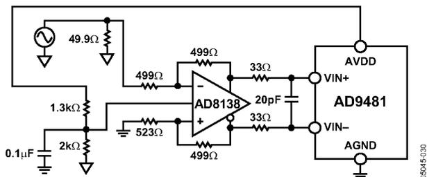
Figure 29. Driving the ADC with the AD8138
