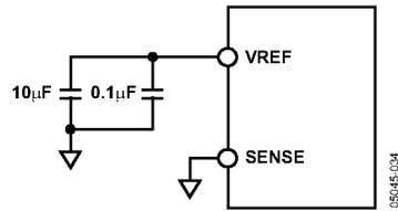
Figure 33. Internal Fixed Reference (1 V p-p)
