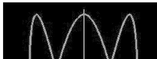
This shows the sine wave 90 degrees out-of-phase with the frequency of the horizontal sine wave three times the frequency of the vertical sine wave.
