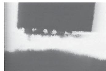
**Figure 15.** Outline of cavitation bubble cloud (the black images below the black rectangle) on the face of a phacoemulsifier (adapted from A. Y. Anis 2003, personal communication, reproduced with permission).
