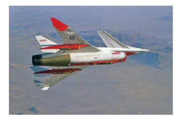
HiMAT research at Dryden was conducted jointly by NASA and the Air Force Flight Dynamics Laboratory, Wright-Patterson Air Force Base, Ohio. Because the planes were controlled from a ground station, experimental technologies and high-risk maneuverability tests could be employed without endangering pilots. The aircraft were flown 26 times during the 3 1/2 year history of the program.
