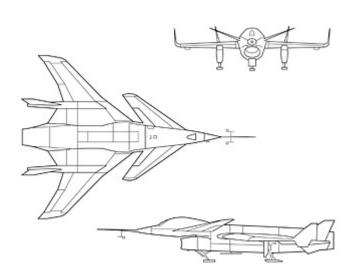
The HiMAT plane's rear-mounted swept wings, digital flight control system, and forward controllable canard made the plane's turn radius twice as tight as that of conventional fighter planes. At near the speed of sound and at an altitude of 25,000 feet, the HiMAT vehicle could substain an 8-G turn (that is, one producing acceleration equal to 8 times that of gravity). By comparison, at the same altitude, an F-16's maximum sustained turning capability is about 4.5 Gs.
