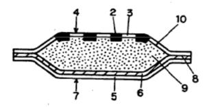
Ohbiki's Figure 1 above depicts a containment bag for a heat generating agent including a non-thermally fused portion of a porous film 2, a thermally fused portion of a porous film 3, a porous film wrapping material 4, a non-woven fabric 5, an air-impermeable film 6, an air-impermeable wrapping material 7, a heat sealed portion 8, a heat generating agent 9, and a through hole 10 (p.18).
