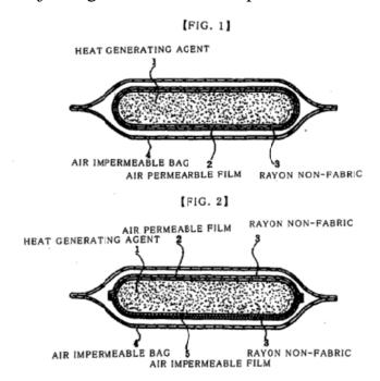
Tsuji's Figures 1 and 2 above depict sectional views of the disclosed warming apparatus including heat generating agent 1, air permeable film 2, rayon non-woven fabric 3, air impermeable bag 4, and air impermeable film 5 (pp. 6-7).
